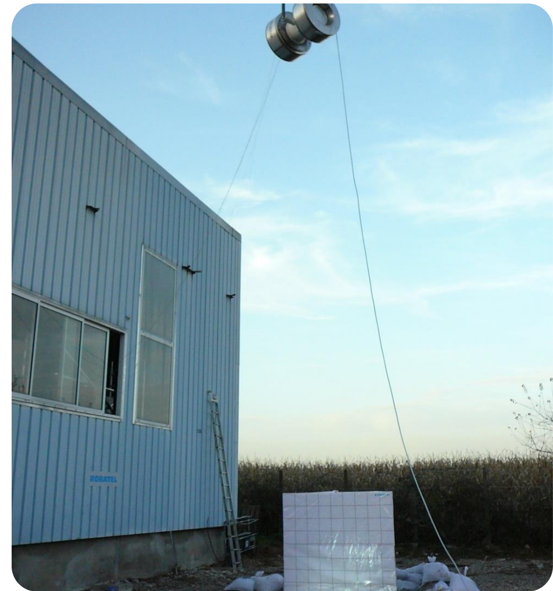
➤ RT100 scale model - 9m drop
