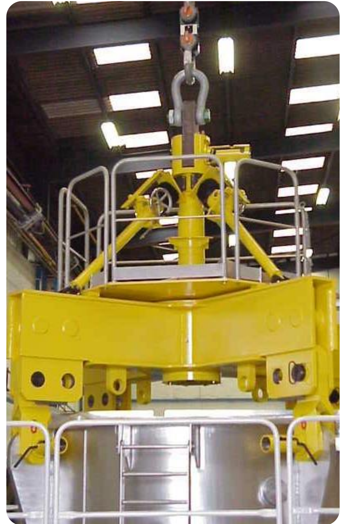
➤ VVP lifting fixture with trim adjusting system – 70 T WLL
