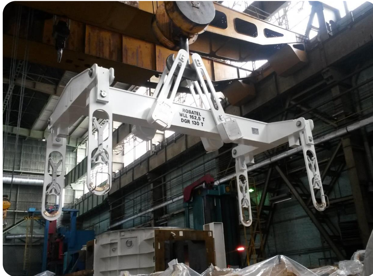
➤ Lifting fixture for a spent fuel cask ANSTO – 130 T WLL
