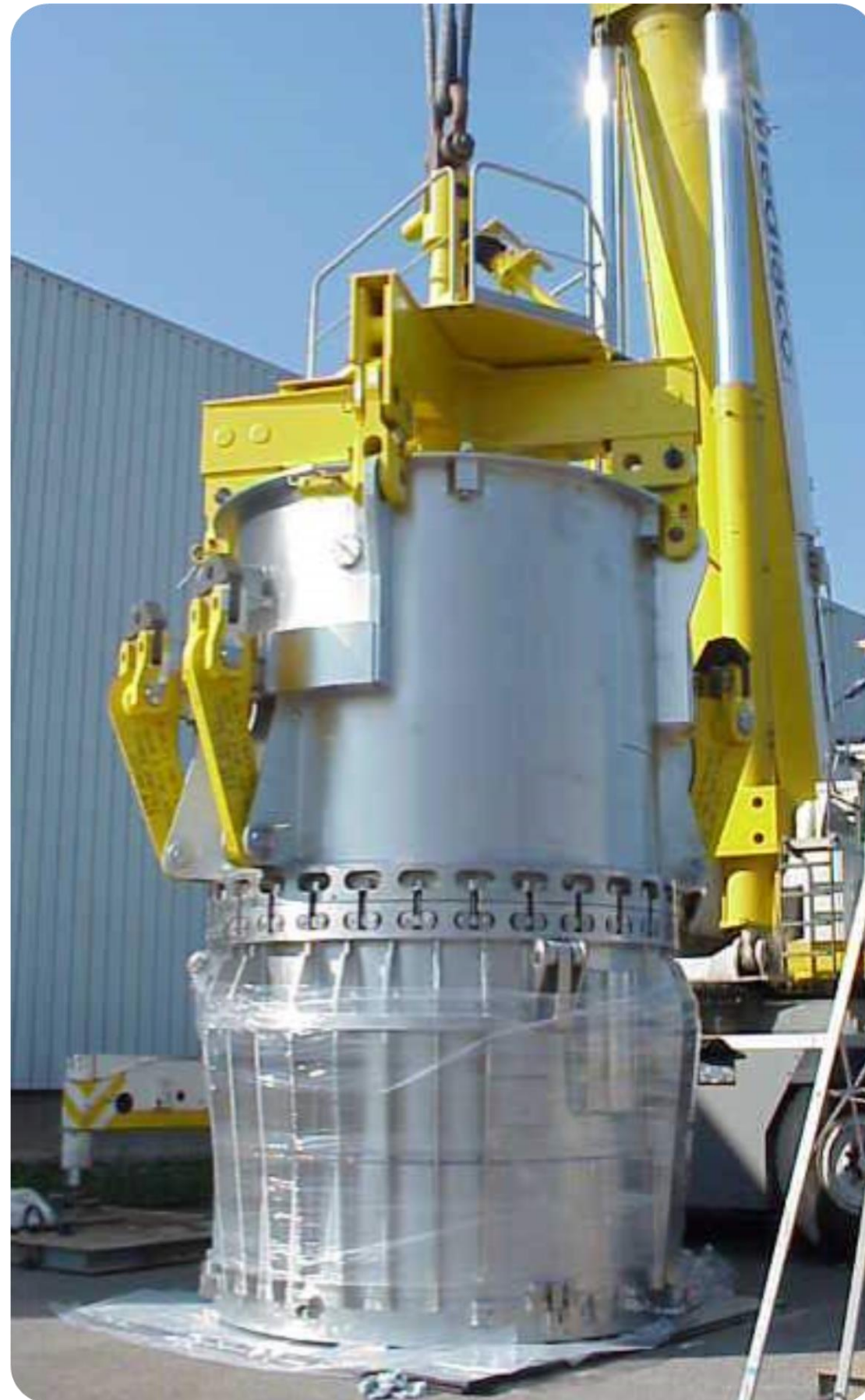
➤ Lead shielded shell VVP - 70 Tons
