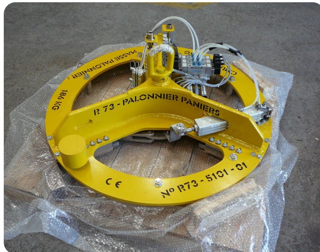
➤ R73 cask pneumatically actuated lifting fixture
