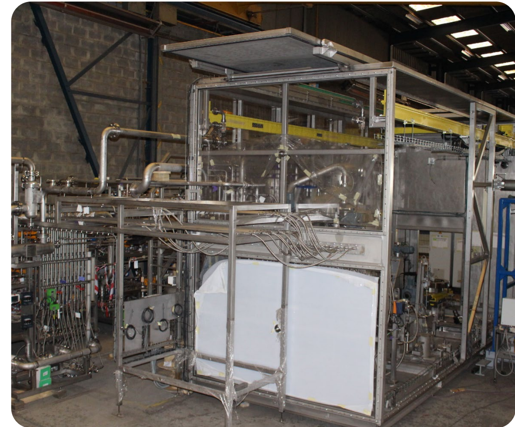
➤ Containment enclosure and in-cell overhead crane
