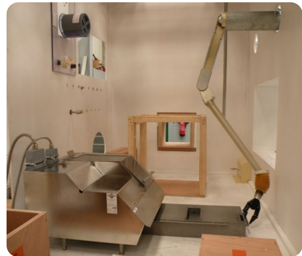
➤ Mockup for ergonomics and accessibility testing
