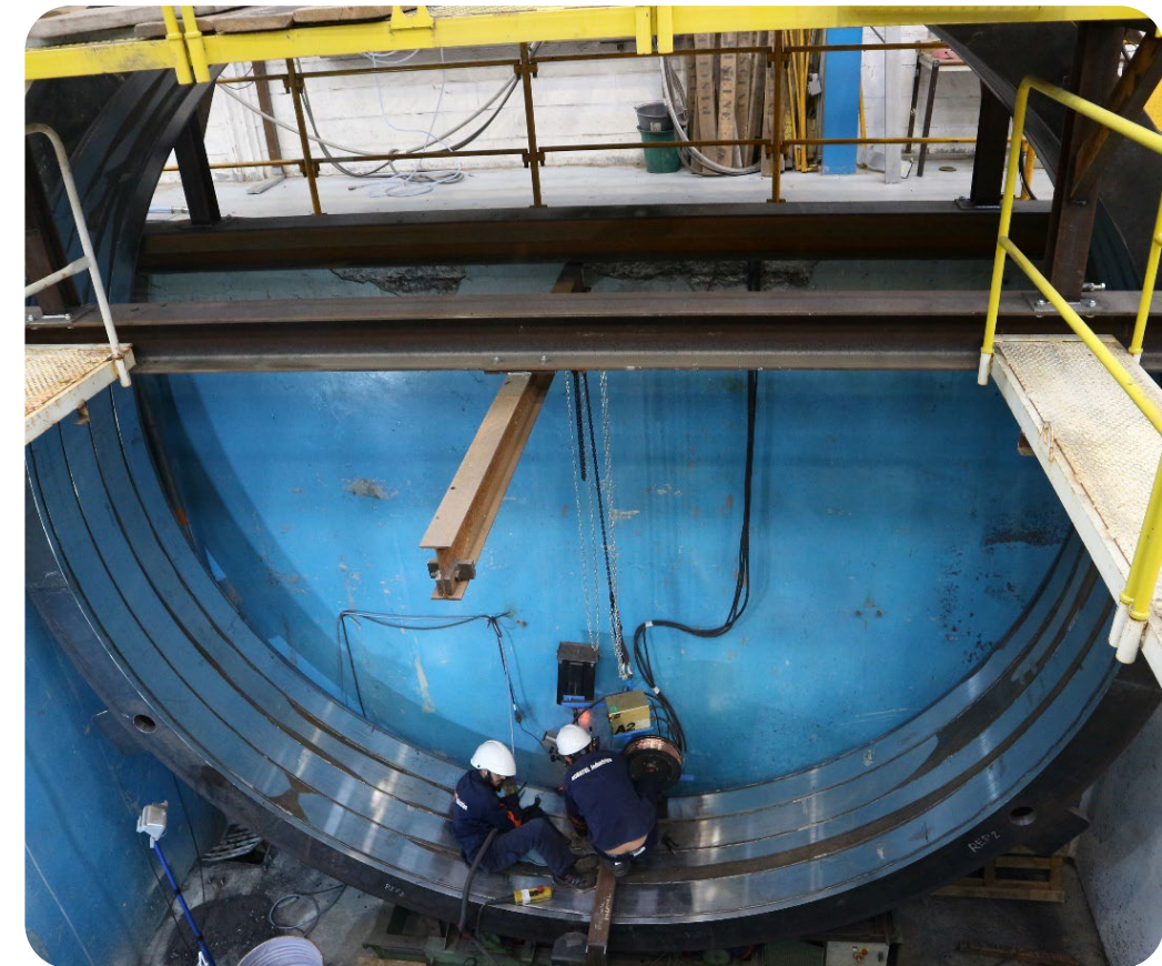
➤ Lifting fixture under fabrication (at ROBATEL Industries in Genas France)
