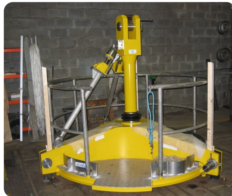
➤ K15 container lifting fixture with trim adjusting system – 90 T WLL
