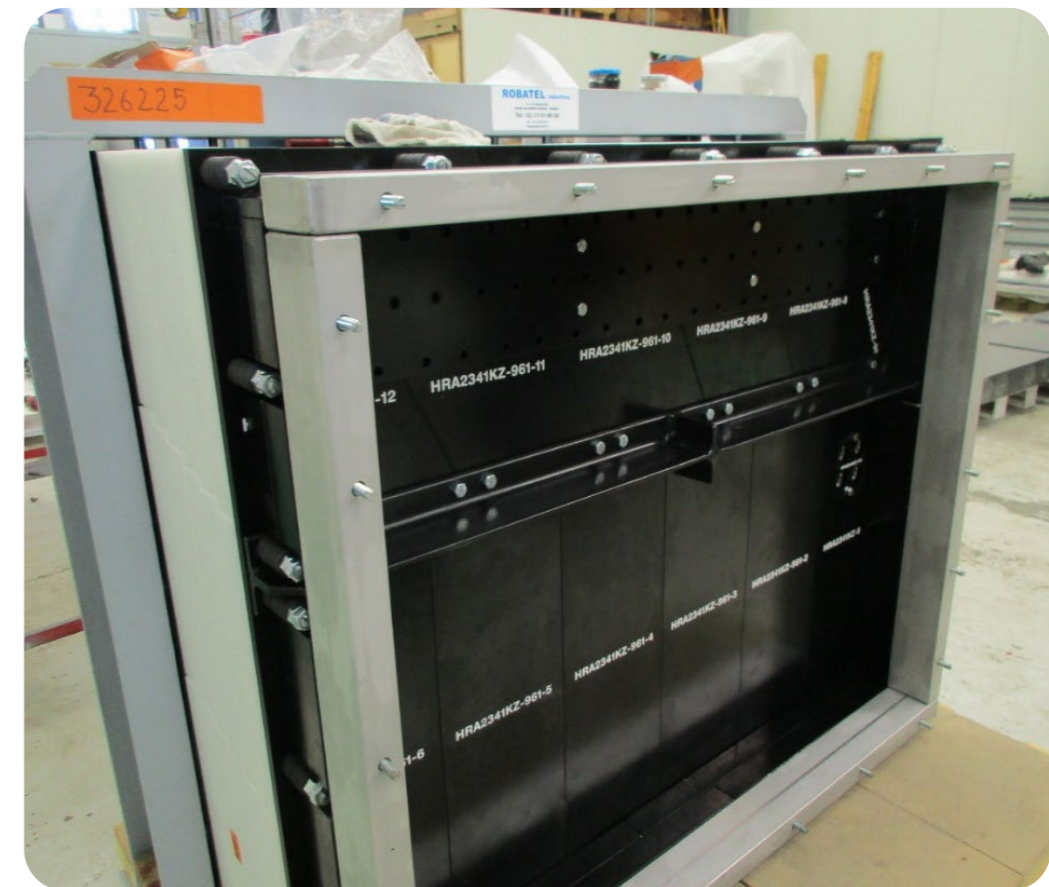
➤ Protections neutroniques Piscine / AEROBALL
